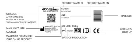
SERIAL NUMBER IN BARCODE FORM SN KTK 007/B/1/BD SERIAL NUMBER
