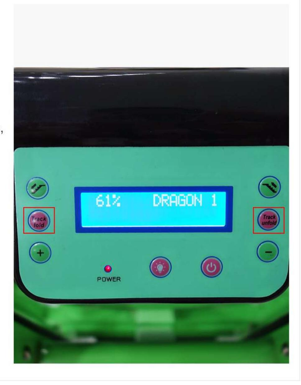
17. Press the red button, make the track stop at any angel to suitable for the stairs of different angel.
